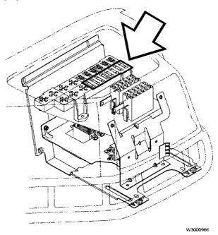
**Note:** Refer to the decal inside the TEC cover for vehicle's exact fuse descriptions and ratings.
