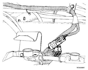
One or two in-line fuses may be used, depending on engine type. For more information on the number of fuses and rating, refer to the VNL, VNM electrical schematic service manuals.
