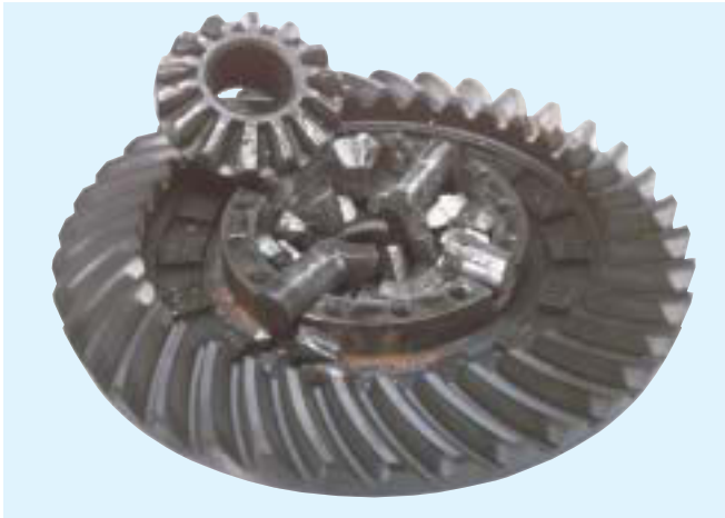
Side Gear - Catastrophic Shock
