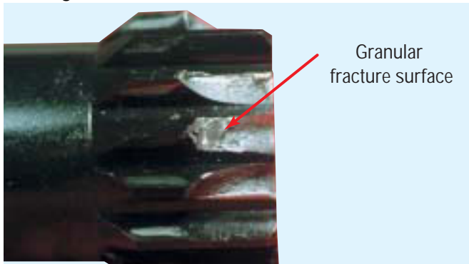
Sliding Clutch - Shock Failure
