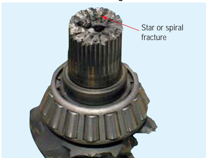
Drive Pinion - Torsional Fatigue Failure
