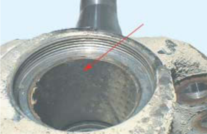
Bushing - Lack of Grease
