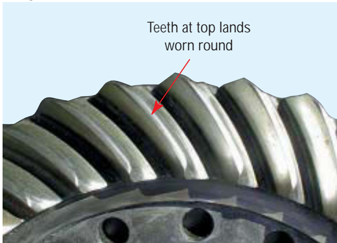
Ring Gear - Low Lube - Crows Foot
