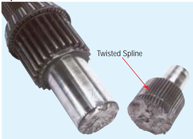
Input Shaft - Torsional Shock Failure
