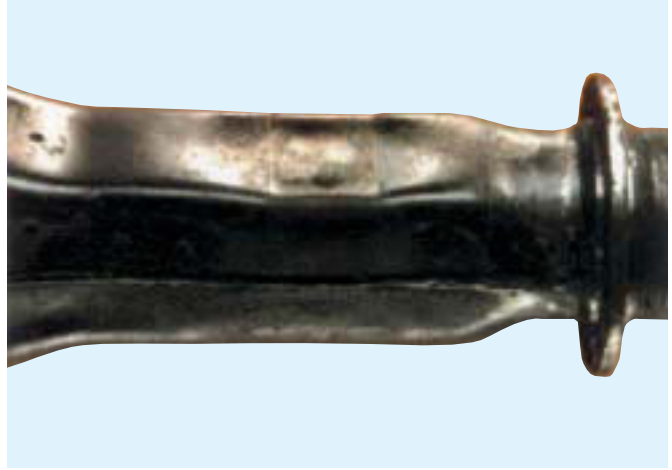
Over-torqued Clamping Hardware
