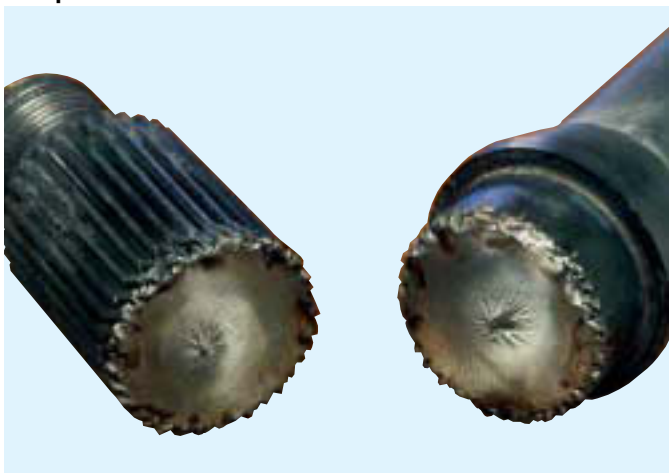
Output Shaft - Torsional Shock Failure
