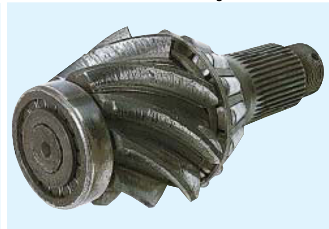
Drive Pinion - Low Lube - Scoring
