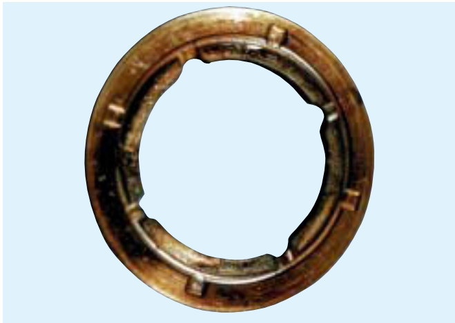
Power Divider Thrust Washer - Lubricant Contamination
