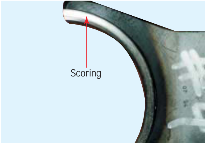
Helical Side Gear Bushing - Lubricant Contamination
