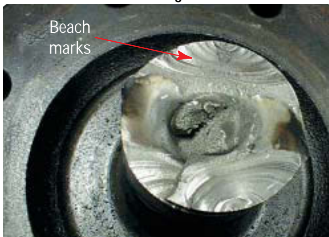
Axle Shaft - Torsional Fatigue Failure
