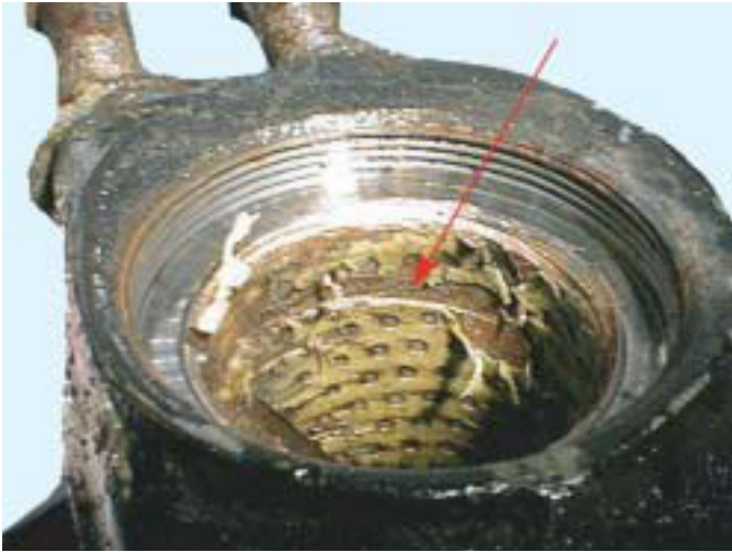
Improper Kingpin Installation
