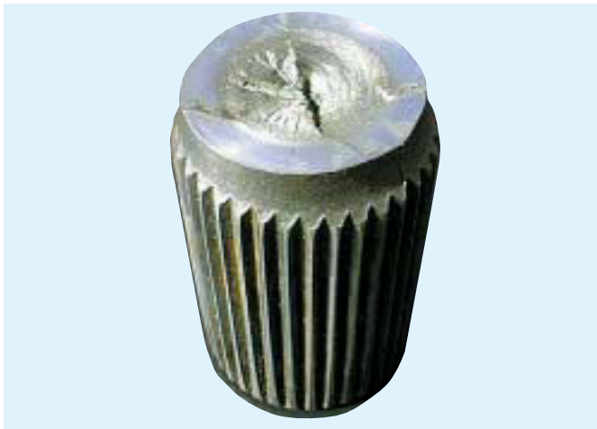
Axle Shaft - Torsional Fatigue Failure
