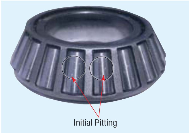
Bearing Cone - Spalling
