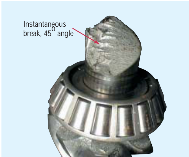
Drive Pinion - Torsional Shock Failure
