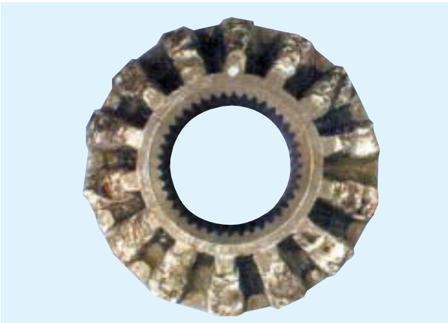
Side Gear - Catastrophic Shock
