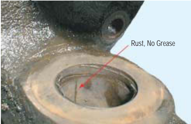
Bushing - Lack of Grease
