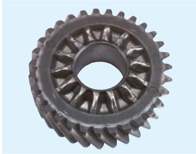
Helical Side Gear - Bushing Burn-Up
