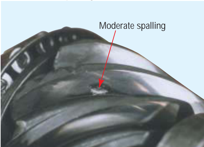
Drive Pinion - Spalling
