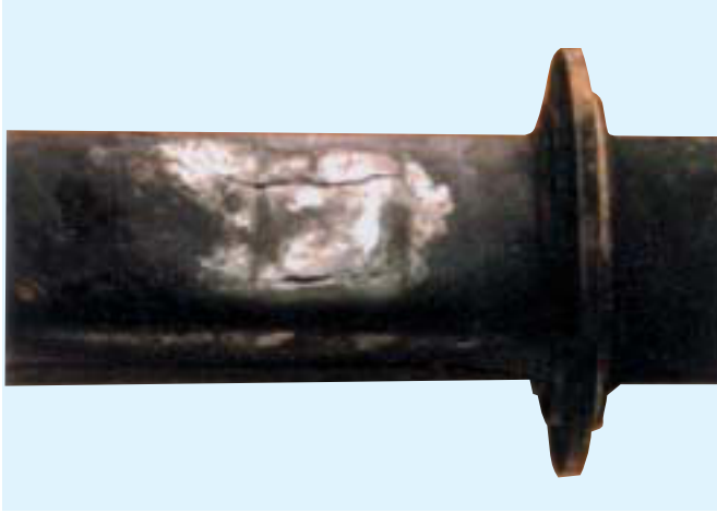
Loose Clamping Hardware
