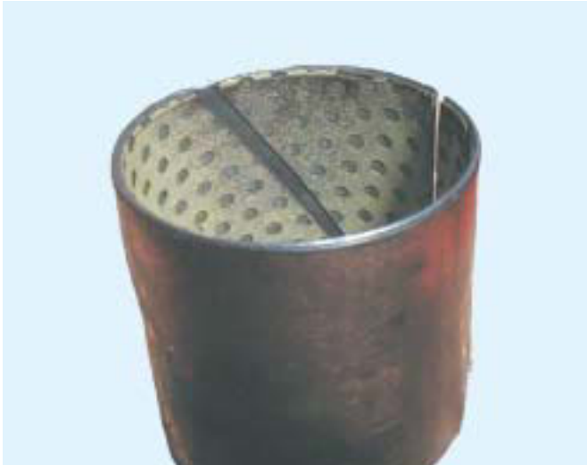
Bushing Worn in One Area Only
