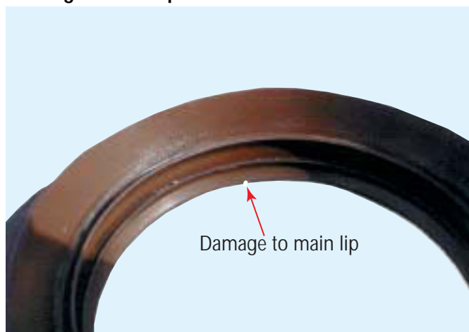
Damaged Seal Lip
