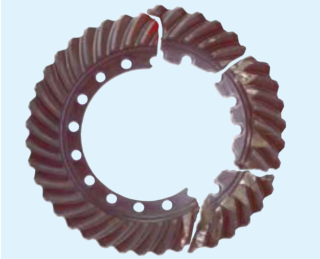
Drive Pinion - Torsional Shock Failure
