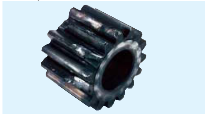
Planetary Gear - Shock Failure
