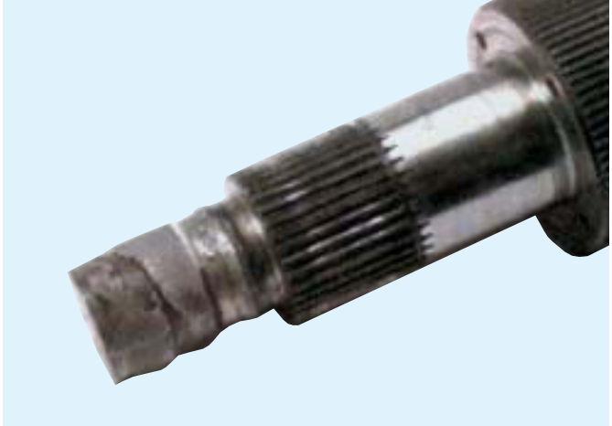
Output Side Gear - Stub-End Bore Galling
