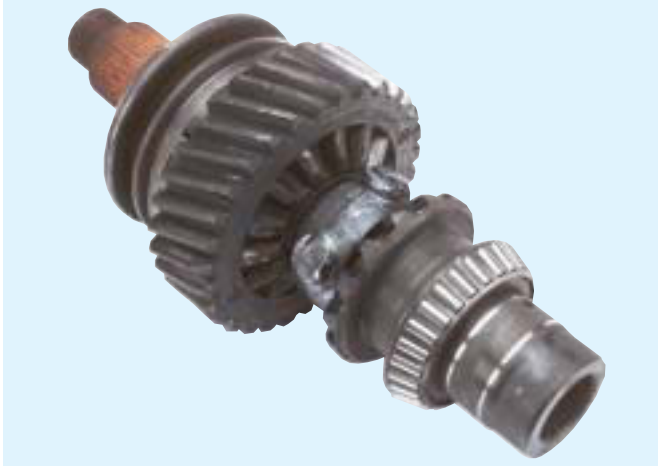
Helical Side Gear - Bushing Burn-Up
