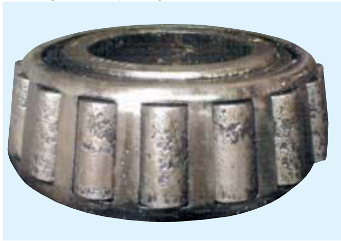
Bearing Cone - Spalling
