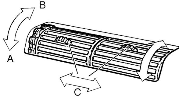
When heating the cab, all vents should be closed. However, the vents on the outer parts of the dash can be used for defrosting the cab door windows. When operating the air conditioning, all air vents should be completely open and the air flow directed upward.
